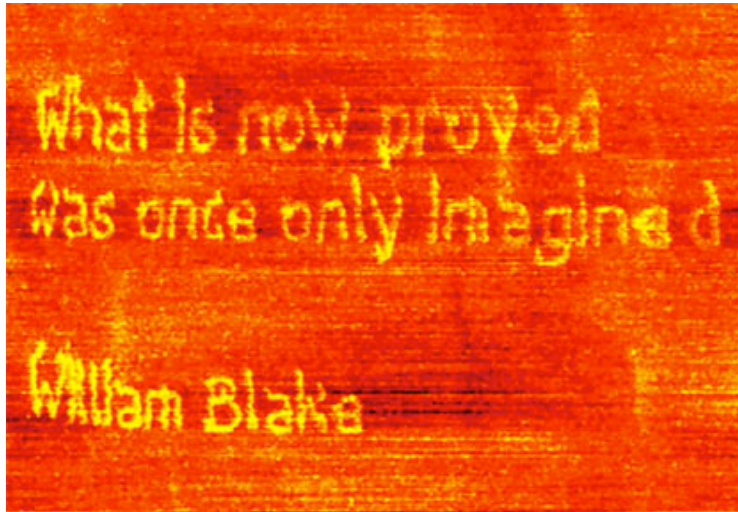
Automated AFM nanografting with mercapto-hexadecanoic acid in a mixed hexanethiol/octadecanethiol SAM
